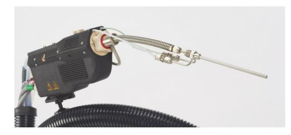
Measuring trace amounts of hydrocarbons in air at 400 Hz.
