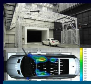
Identification of pressure distribution around the vehicle by means of combination of multiple arrays
