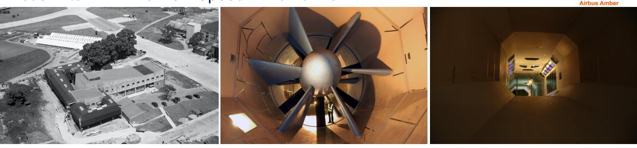
The Airbus Filton LSWT is of the Göttinger type, closed return circuit design, powered by an rpm controlled motor.Construction of the wind tunnel commenced in 1954 and was commissioned in **1956**.Test section dimensions: **3.65m** x **3.05m** x **8.5m** (12 ft x 10 ft x 28 ft) with corner fillets which reduce the cross section to octagonal.Power: **1.6 MW**Contraction ratio: **6.65**Speed range: **0 to 97m/s**
