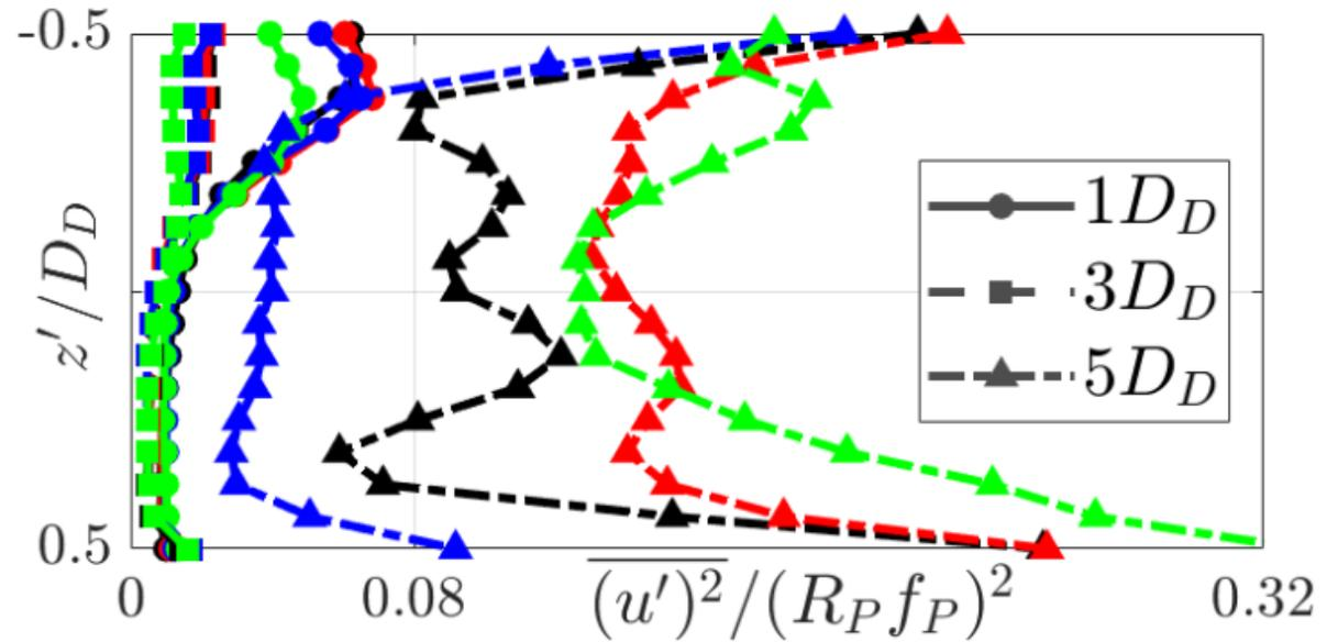
Figure 12: Mean velocity and Reynolds stress profiles for each blockage element (1 (35%), 2 (50%), 2B (50%, holed), and 3 (65%)).
