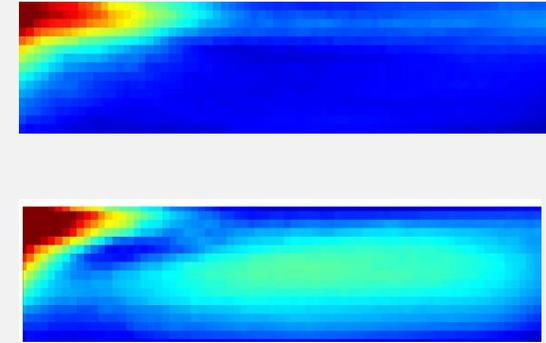
The duct **ingests two discrete structures**, the root vortex and the vortex sheet, and their associated energies make the **blade passing frequency dominant** within the entrance region of the duct.
