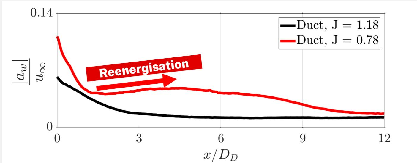
The duct **ingests two discrete structures**, the root vortex and the vortex sheet, and their associated energies make the **blade passing frequency dominant** within the entrance region of the duct.
