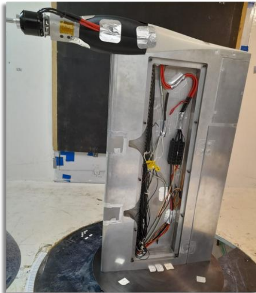
Wing-propeller model internal wiring.
