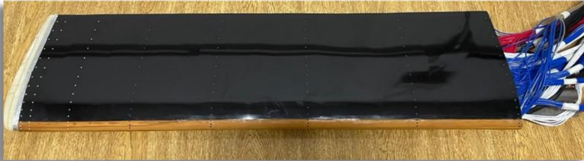
Wing model with a conventional tap layout.
